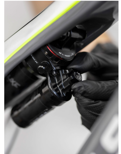
Shock compression adjustment
