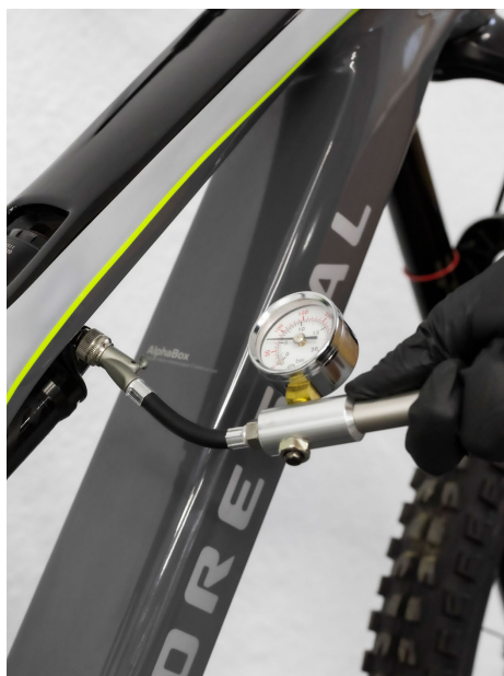
Adjust the air pressure in the shock
