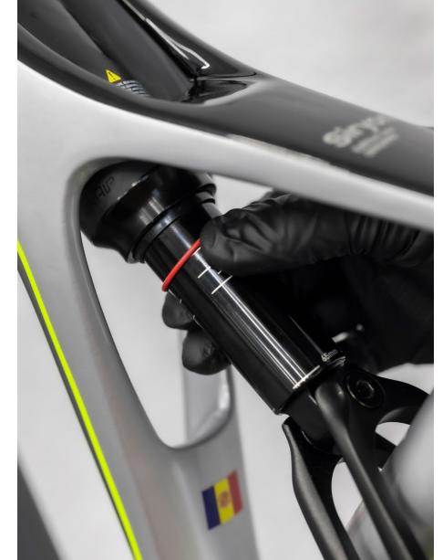
Set O-ring on the shock
