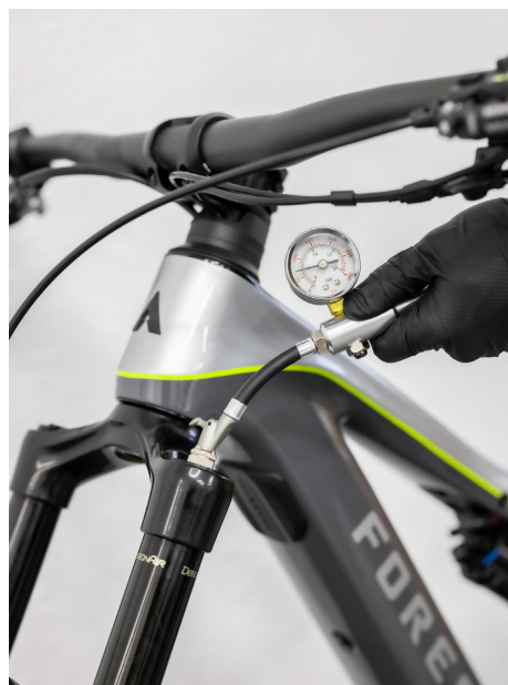
Adjust the air pressure in the fork
