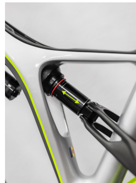
Cycle shock through the travel
