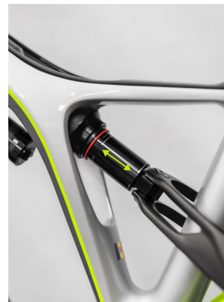
Cycle shock through the travel
