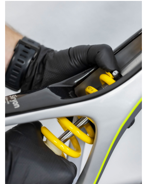
Coil shock preload adjustment
