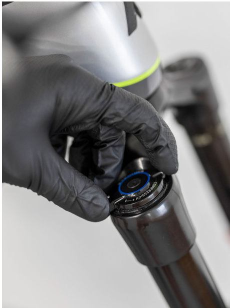
Fork compression adjustment
