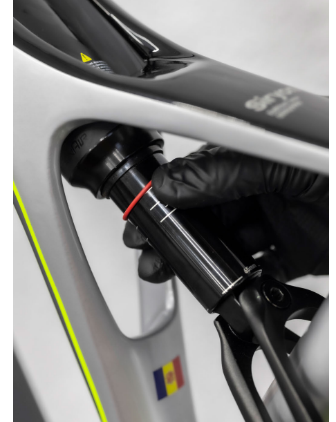
Set O-ring on the shock
